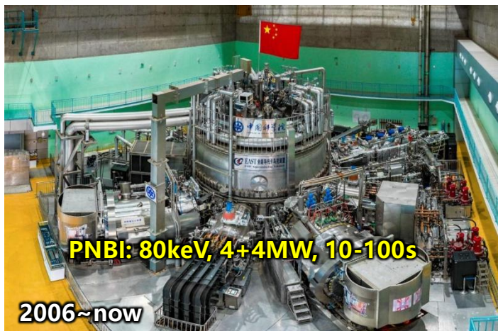
EAST | First full superconducting tokamak
