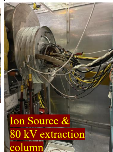
Ion Source Racks Floating at 80 kV
