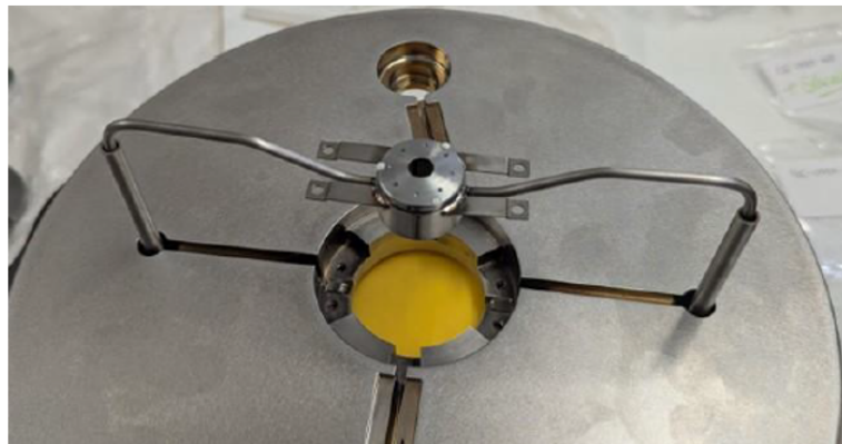
Figure 8: Caesium collar and new flange
