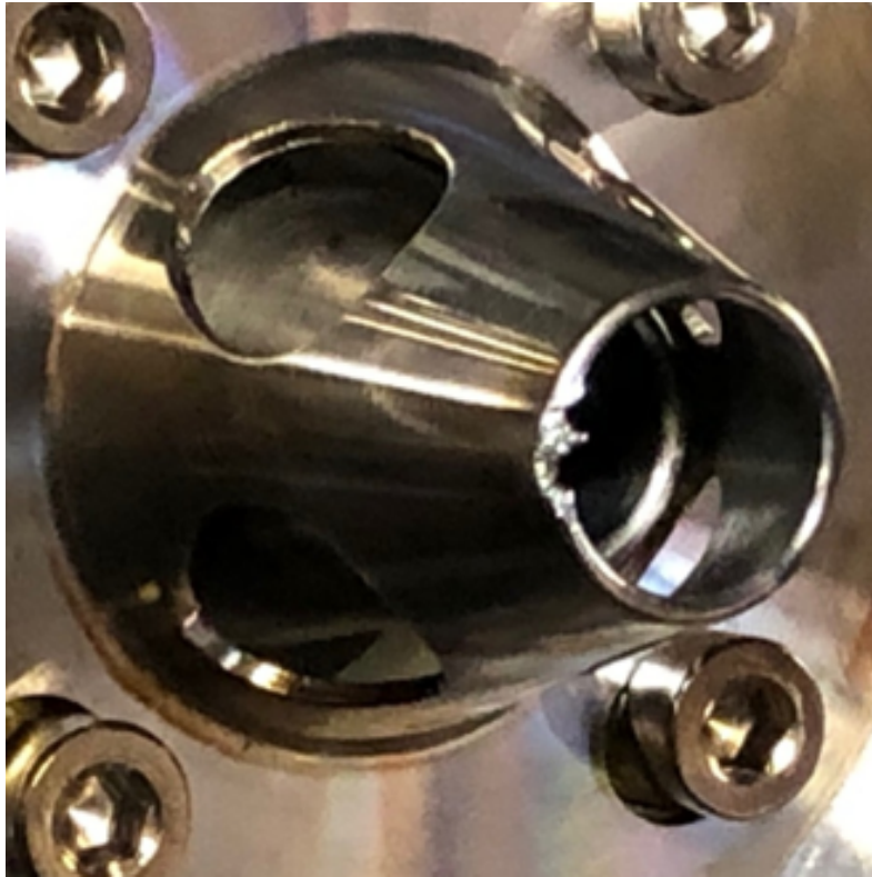
Figure 7: Damage to protection electrode from secondary electrons
