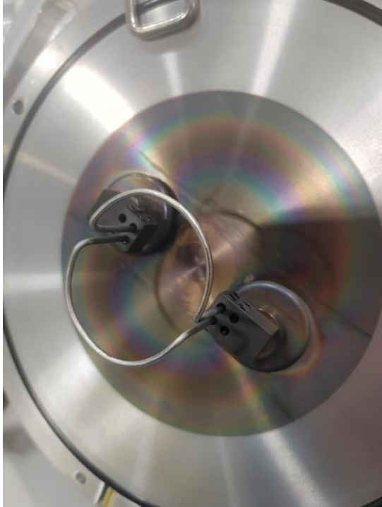
1. Tantalum Filament heats the gas
