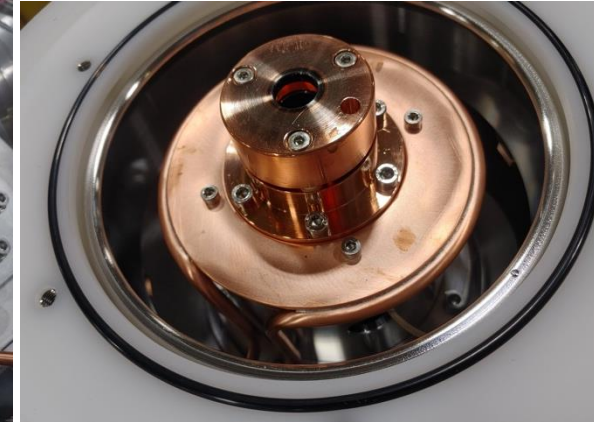
4. Magnets filter electrons and allow for H^- production via charge-exchange. Voltage applied to electrode to transport + beam (if needed).
